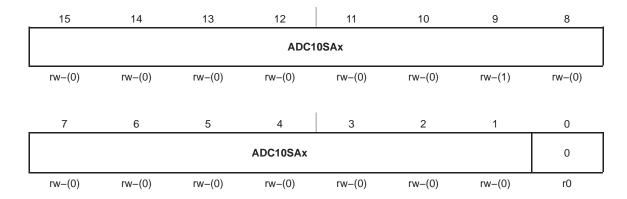
ADC10SAx Bits ADC10 start address. These bits are the start address for the DTC. A write
